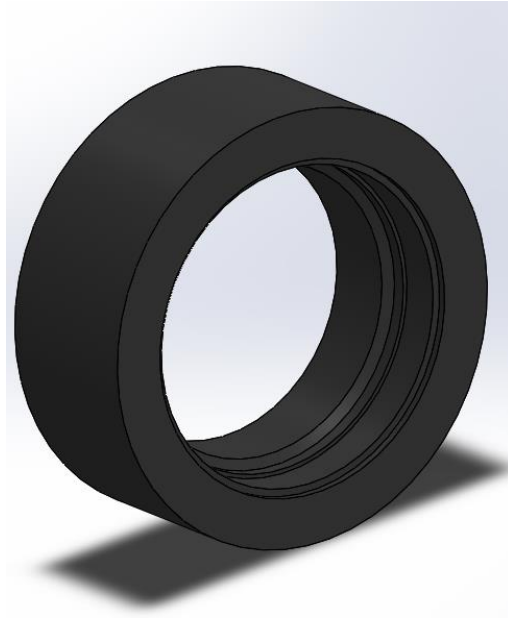
Figure 18: Using the Revolve feature around a Circular Axis
